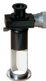
Standard microscope (0.01 mm high resolution microscope with 6 mm drum scale)
